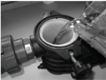
Prime the pump (if not risk of dry running). WARRANTY LOSS!!!
