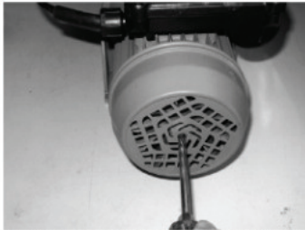
In order to avoid mechanical seal blocking, turn the shaft trough the motor fan before starting up or after extended unuse!
